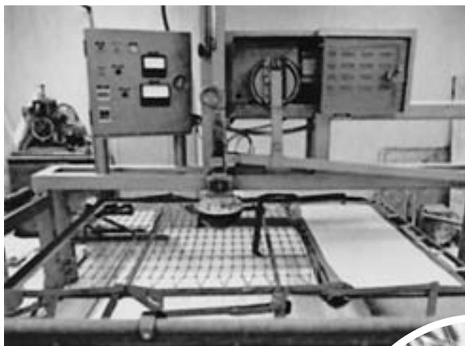
Above left: Using a Cornell Tester developed by Cornell University, Leggett & Platt tested its sofa sleeper mechanism by maintaining pounding pressure on the unit all day long.
